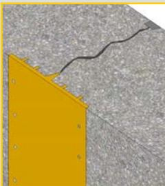
Kryton's Crack Inducing Waterstop creates a controlled crack and then introduces Krystol technology through an externally placed waterstop that ensures permanent waterproofing protection.
