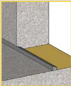
Krystol technology delivered through a slurry treatment and external waterstop that ensures permanent waterproofing protection.
