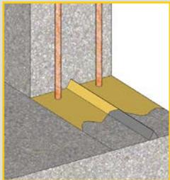
Krystol technology delivered through an internally placed, triangle-shaped waterstop and a slurry treatment that ensures permanent waterproofing protection.
