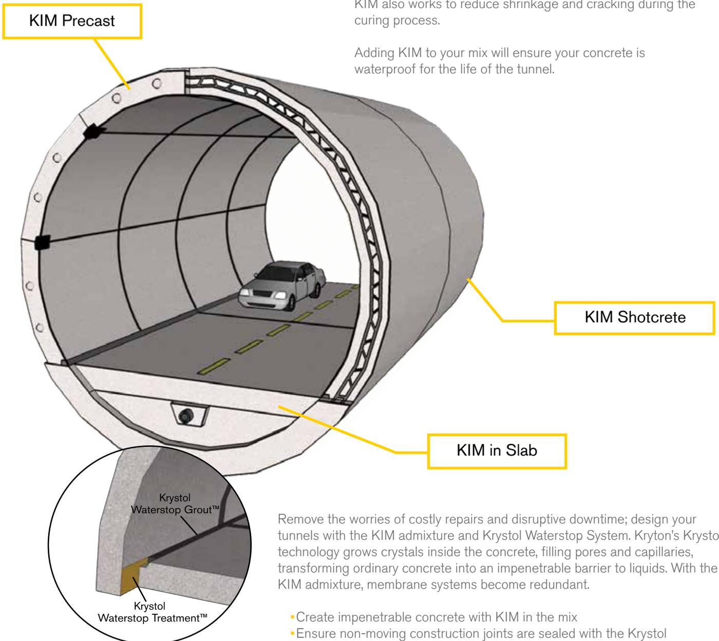
Remove the worries of costly repairs and disruptive downtime; design your tunnels with the KIM admixture and Krystol Waterstop System. Kryton's Krystol technology grows crystals inside the concrete, filling pores and capillaries, transforming ordinary concrete into an impenetrable barrier to liquids. With the KIM admixture, membrane systems become redundant.
