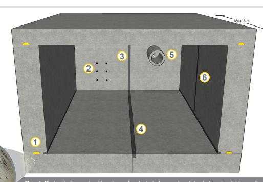
Krystol® chemically reacts with water and un-hydrated cement particles to form insoluble needle-shaped crystals that fill capillary pores and micro-cracks in the concrete and block the pathways for water and waterborne conteminants. Any moisture introduced over the lifespan of the concrete will initiate crystallization, ensuring permanent waterproofing protection.
