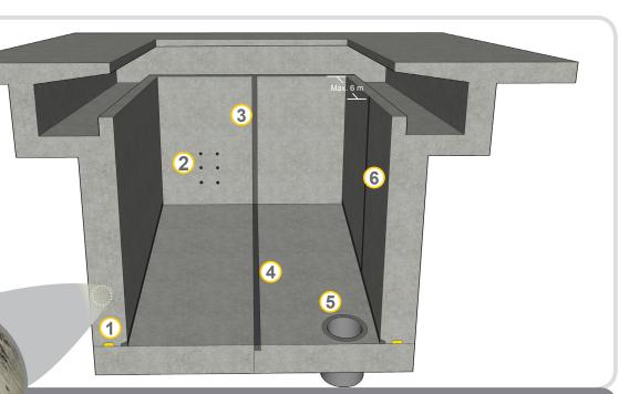
Krystol® chemically reacts with water and un-hydrated cement particles to form insoluble needle-shaped crystals that fill capillary pores and micro-cracks in the concrete and block the pathways for water and waterborne conteminants. Any moisture introduced over the lifespan of the concrete will initiate crystallization, ensuring permanent waterproofing protection.
