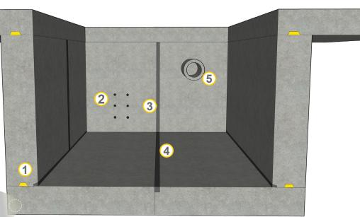
**Krystol**<sup>®</sup> chemically reacts with water and un-hydrated cement particles to form insoluble needle-shaped crystals that fill capillary pores and micro-cracks in the concrete and block the pathways for water and waterborne conteminants. Any moisture introduced over the lifespan of the concrete will initiate crystallization, ensuring permanent waterproofing protection.
