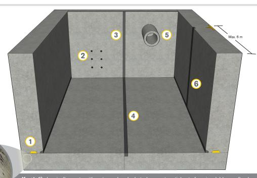
Krystol® chemically reacts with water and un-hydrated cement particles to form insoluble needle-shaped ensuring permanent waterproofing protection.
