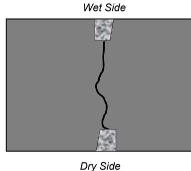
**IMPORTANT:** The control joint components must be directly across from each other. If they are offset, cracks may form outside of the keyways.
