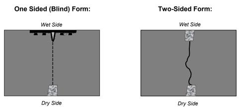
**IMPORTANT:** The control joint components must be directly across from each other. If they are offset, cracks may form outside of the keyways.
