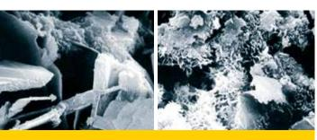
Regular mortar (Left) VS Krystolized mortar (Right)
