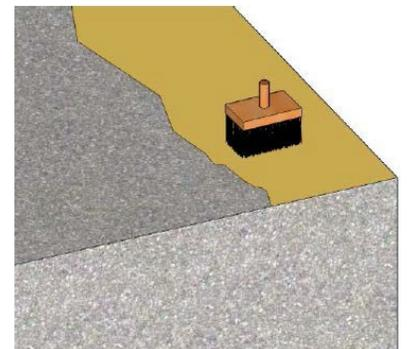
3. Use a concrete brush to coat the entire joint. Ensure the Treatment fills all surface voids and is at about 1 mm (40 mil) thick. Do not allow Treatment to build up on reinforcement. **NOTE:** After mixing, the material may thicken in the pail. Do not add more water. Remixing will make the material easy to spread again.
